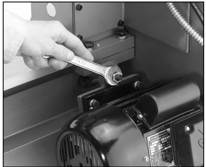
Figure 16. Tension nut shown.
